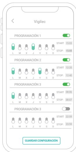
It has four independent timers to program the use of the equipment, click on the parameter to change it.
