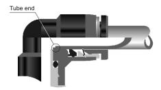
(3) On completion of fitting, make certain that the tube does not come out at your pulling.
